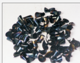
Chip feature after drilling
