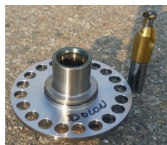
After drilling & back chamfering
